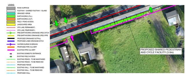
Figure 4-5 Close up of boundary details from EIAR Figure A4.13 with Legend included
